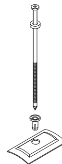
Drive screw with sealing washer, plate and plug
